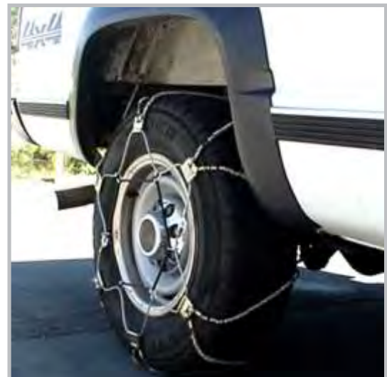
Glacier Light Truck V-Trac Cable Shown
