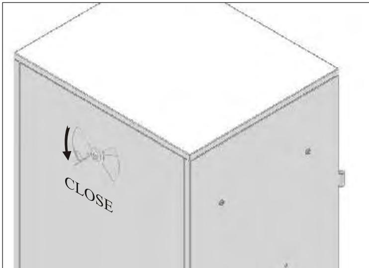
The damper allows adjustment of exhaust air while cooking. Less exhaust air will allow for the smoker to burn hotter and keep the flavoring smoke inside the smoker.
