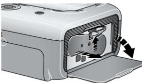
To remove the color cartridge, open the color cartridge door, then push up on the green lever and slide the cartridge out.
