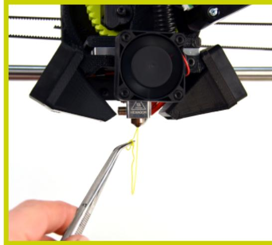
**9C** Wait ten seconds for the filament to cool, then remove the extruded filament with the included tweezers.
