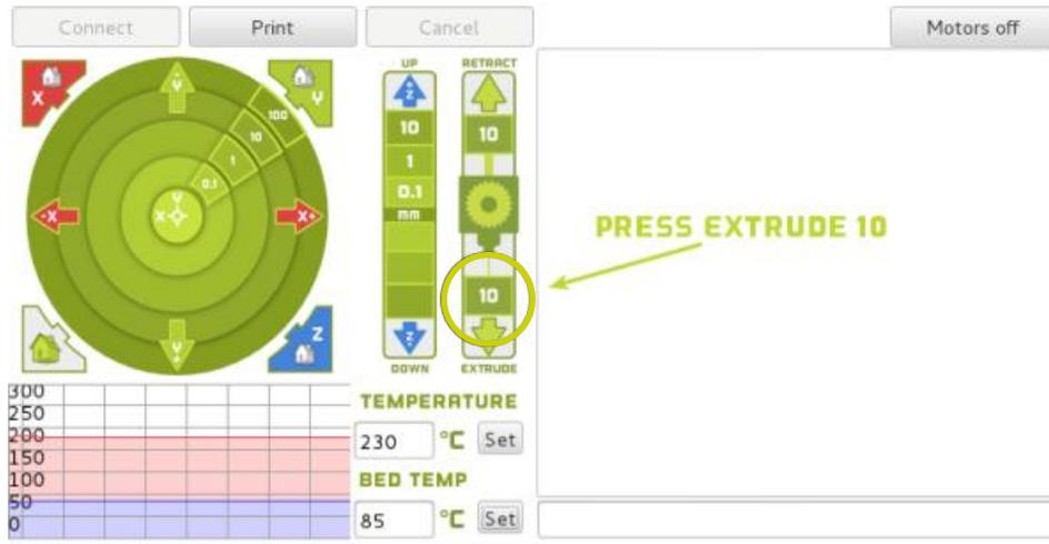
**9B** If you do not see filament coming through the nozzle and the drive gear stops moving, click the **Extrude 10** button once more and wait. Repeat as needed until you see consistent and repeatable extrusion.
