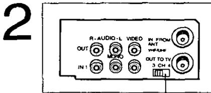
**2** Tune to VCR output channel. Tune TV to CH3 or CH4. (Same as back of VCR)
