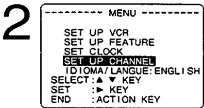
**Display SET UP CHANNEL.**
