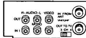
Slide the VCR Channel selector switch to the channel number not used by local broadcast companies (CH3 or 4).
