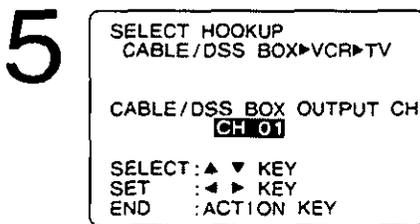
**5** Select cable box or DSS receiver output channel. 1) Press ▲▼ to select. 2) Press ▶ to enter.
