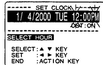
4) Press ▲▼ and ◀▶ to select and set the date, time, and DST (Daylight Saving Time).
