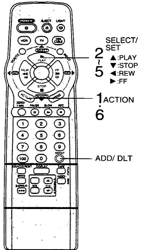
**\*Important:** If the remote control POWER, ACTION, PROG, CH▲/▼, INDEX, TAPE POSITION, or ADD/DLT button does not work when pressed, press the VCR button on the remote and try the button again.
