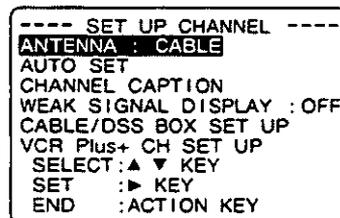
3) Press ▲▼ to select "ANTENNA," then press ► to set your antenna system (TV or CABLE).
