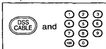
Hold down DSS/CABLE and enter code with NUMBERED keys.
