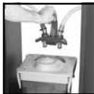
3. Gently disengage the Quick Disconnect Valve from the top of the Blue Motor Housing.
