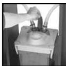
2. Lift up on the Quick Disconnect Valve.
