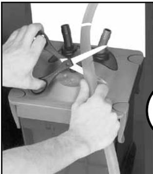
Note: It is very important NOT to cut the tubing too short. If the tubing is cut too short it creates tension on the quick disconnect valve, and the filter may leak. Also, leaving the tubing too long may prevent the filter from priming and greatly reduce waterflow.
