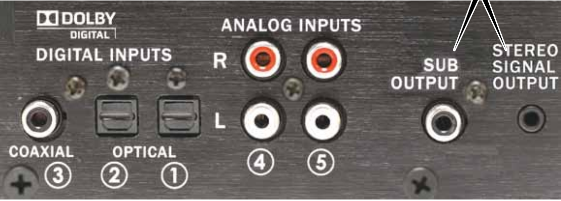
SoundBase Back Panel Inputs and Outputs
