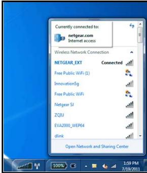
**Tip:** You can use any WiFi network manager utility on a computer or tablet to find and connect to the extender wireless network.
