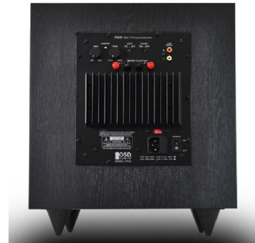
Amplifier Plate, Back panel featuring gain and variable frequency controls
