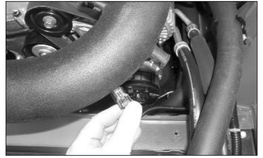
26a. On vehicles equipped with an air temperature sensor, position the air temperature sensor wiring harness on the intake tube for best fit and mark the position on the intake tube with a marker for drilling.
