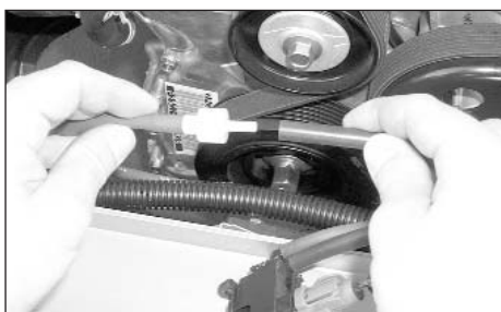
15. On vehicles equipped with air injection pump, attach the provided 4mm(short) vacuum hose to the check valve.
