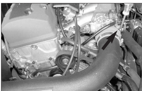
26. Install the K&N intake tube and secure the hump hose to the throttle body as shown.
