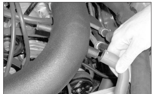
28. On vehicles equipped with air injection pump, attach the air injection hose to the fitting on the K&N intake tube.
