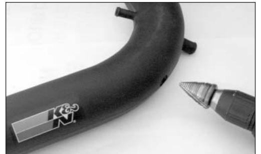
26b. Remove the intake tube from the vehicle and drill a 5/8" id hole in the tube at the position indicated in the previous step.
