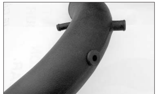
26c. Install the provided grommet into the hole drilled in the K&N intake tube as shown.
