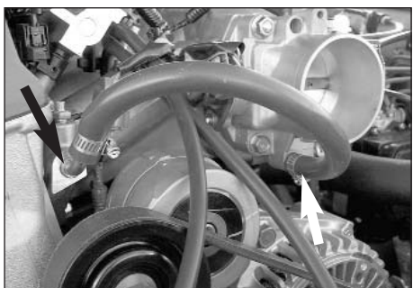
18. Attach the provided 1/4" reinforced hose to the fitting on the intake manifold and the fitting on the underside of the throttle body.
