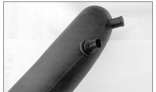
26d. Remove the air temperature sensor from the stock intake tube and install it into the grommet installed in the K&N intake tube in the previous step as shown.
