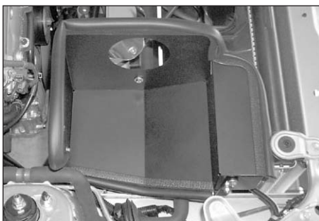
24. Using the provided hardware, install the heat shield assembly and secure the brackets to the original air box mounting locations.
