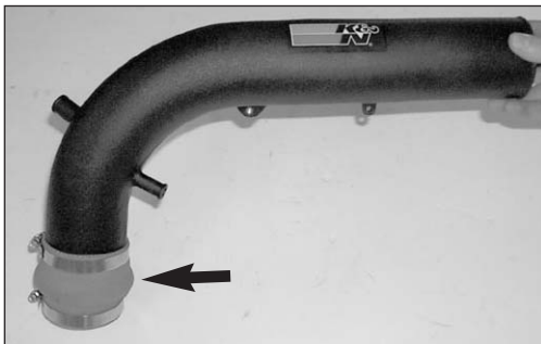
25. Install the silicone hump hose with provided hose clamps, onto the K&N intake tube as shown.
