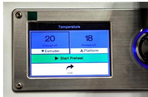
13. If the button under the Extruder and Platform reads Start Preheat, use the control wheel to highlight the **Start Preheat** entry, then press it to start preheating the extruder and build platform. The button will change to read Stop Preheat and the Extruder and Platform buttons will read the actual temperatures.
