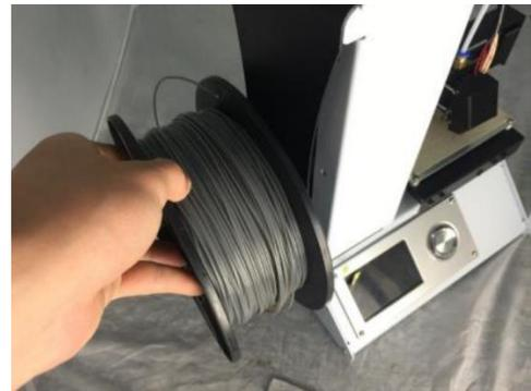
17. While squeezing the lever on the Feed Mechanism, insert the filament and push it into opening. Keep pushing until you feel resistance as it hits the extruder. Release the lever on the Feed Mechanism.
