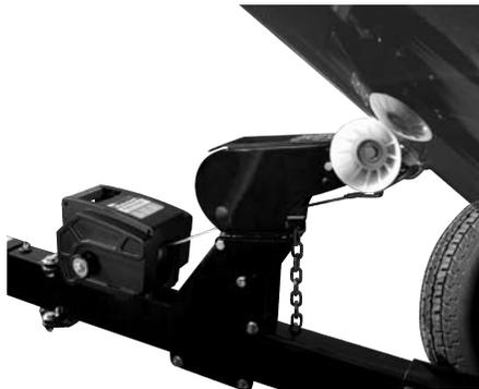
Your winch can generate 2,000lbs of pulling force so be sure that the mounting site selected can withstand a load well in excess of the 2,000lbs pulling force.
