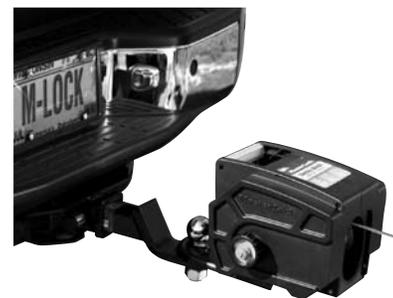
2. Attach the winch adapter mounting plate assembly to your trailer hitch, by inserting the trailer hitch ball through the shaped hole in the adapter mounting plate.
