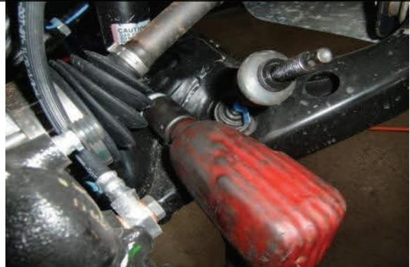
Disconnect and remove lower shock bolt and nut.
