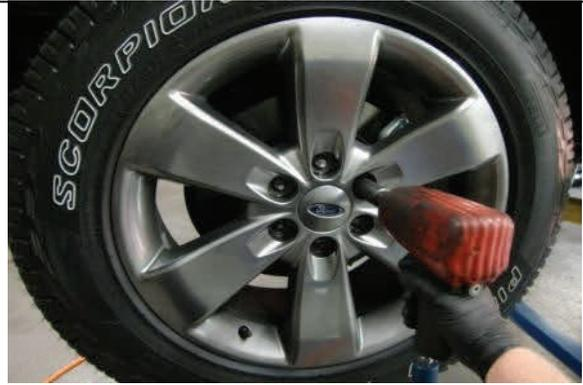
Remove front wheels/tires, support suspension with jack.
