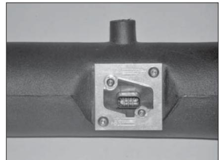
23. Secure the mass air sensor assembly onto the new K&N® intake tube with the provided hardware as shown.
