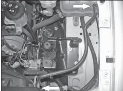
17a. Loosen the coolant recovery hose, hose clamps, and then remove the factory recovery hose shown. Be sure to catch any coolant, which flows out of the radiator during hose removal. **NOTE: Be sure to let the engine cool completely before removing the overflow hose or hot coolant will escape from the radiator and injury or damage may result.**
