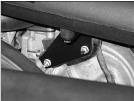
28. Connect the new intake tube to the bracket with the provided hardware as shown.
