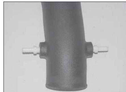
24. Install the provided NPT fittings into the intake tube as shown.
