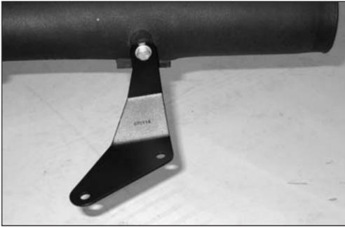
25. Install the tube mounting bracket (070118) onto the K&N® intake tube as shown with the provided hardware.
