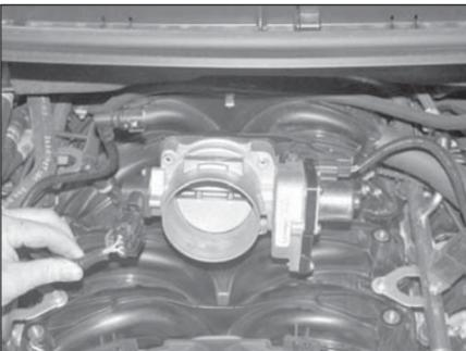
14. Reconnect the throttle body motor and TPS electrical connections.
