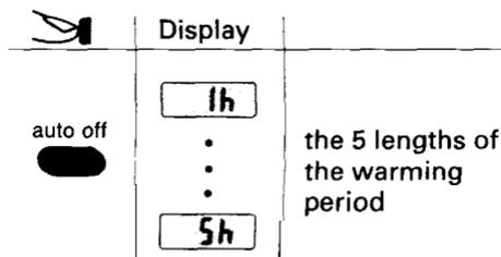
Upon making your selection, the clock time will reappear in the display window after approximately 4 seconds. The automatic shut-off can be adjusted at any time.
