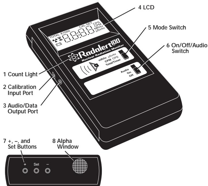
The Radalert 100 counts ionizing events and displays the results on the liquid crystal display (LCD) (4). You control which unit of measurement is shown by using the mode switch.
