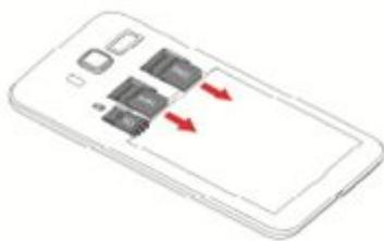
5 the memory card is removed from the card slot, as shown below.
