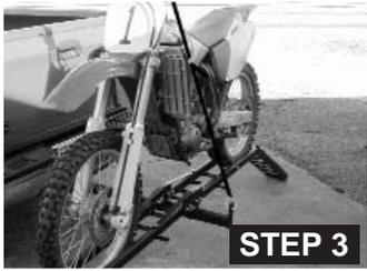
Secure motorcycle with 2 ratchet style straps (not included). Put one of the safety pins into upper hole passing through the spokes of the front wheel. Secure with a clevis pin. **See FIG 5**
